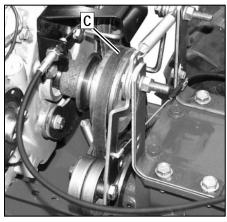
Figure 5-9: Forward clutch belt. (C, Left-side view, no belt cover.)
